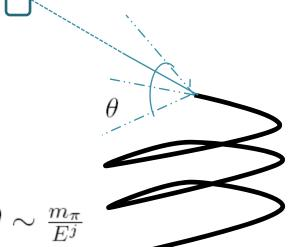
Emission cone with opening angle:  $heta \sim \frac{m_\pi}{E^j}$
