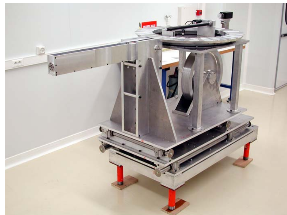
"Carousel" brick dispensing and storage system
