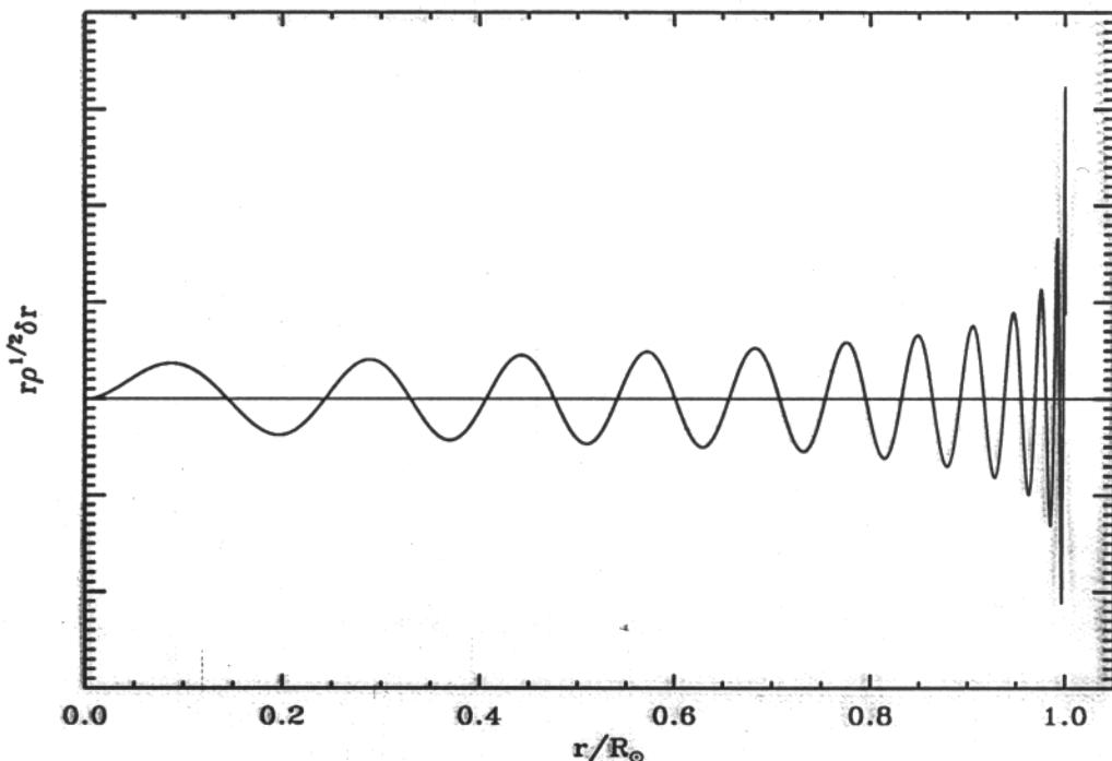
Gravity modes: sensitivity to the nuclear core, 75% from the nuclear core
