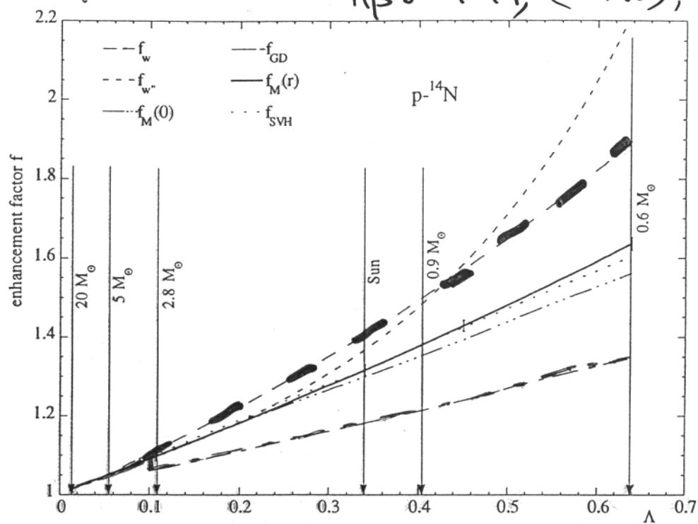
FIG. 3.—Comparison of the screening factors given by the various formalisms for the ( $p, {}^{14}\text{N}$ ) reaction, in central stellar conditions, vs. the screening strength parameter  $\Lambda$ ;  $f_w$  is S54 WS,  $f_{w''}$  is the extended WS,  $f_M(0)$  is Mitler's prescription,  $f_{SVH}$  and  $f_{GD}$  are respectively SVH and GDGC screening, and  $f_M(r)$  is enhancement factor obtained with radial-dependent formalism.
