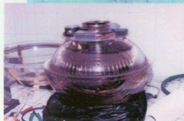
An Optical Module (i.e. a 15" PMT with a HV power supply, inside the protective glass housing)
