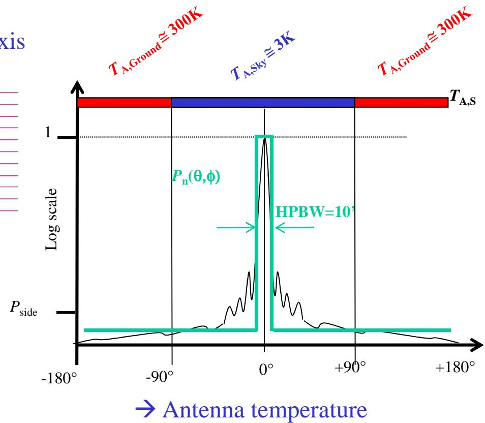
$$T_A(\theta_0, \phi_0) = \frac{\iint T_{B,S}(\theta, \phi) P_n(\theta, \phi) d\Omega}{\iint P_n(\theta, \phi) d\Omega}$$
