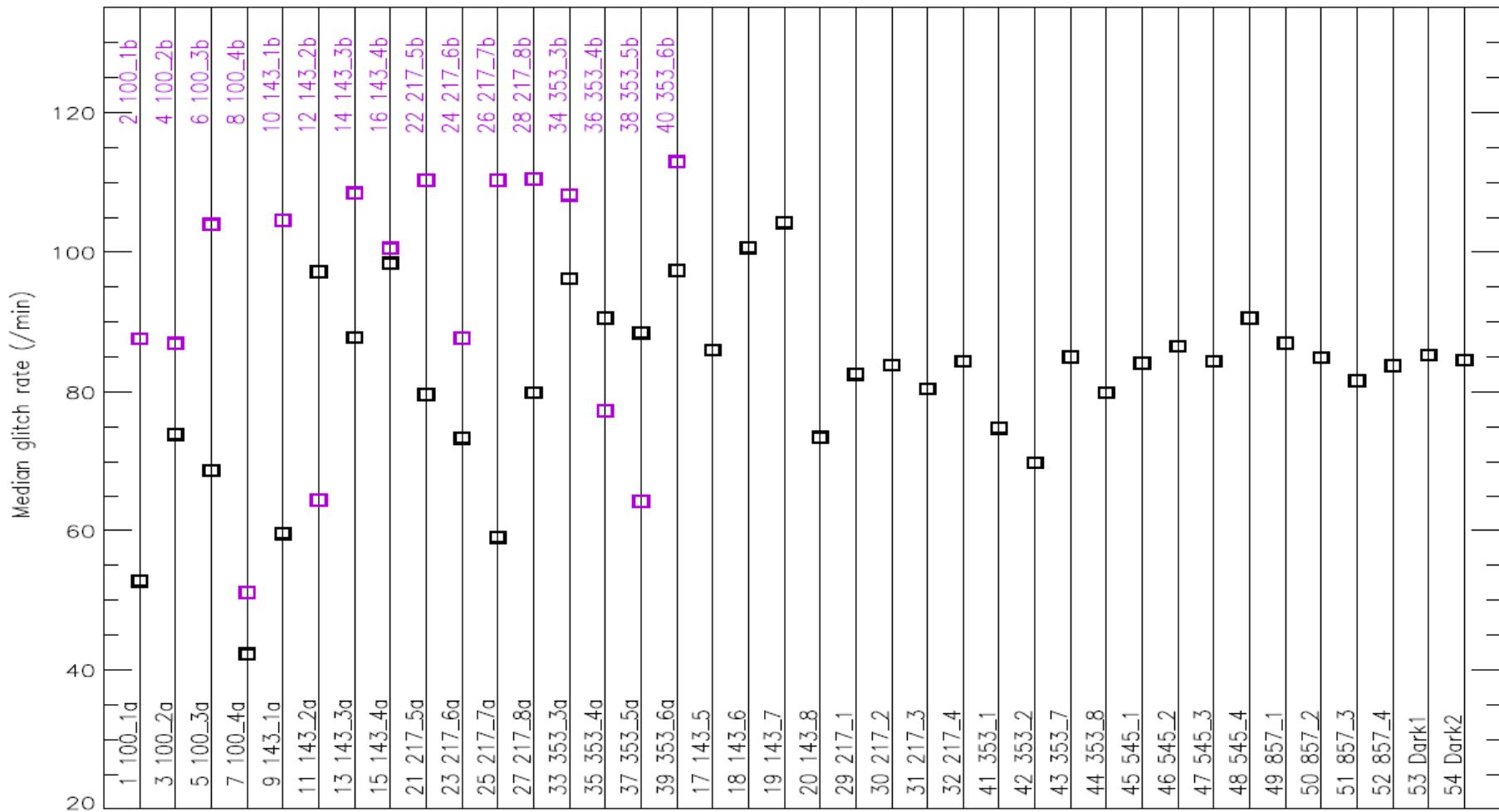
**Figure 19.** Glitch rate of all HFI bolometers. An average over the first sky survey has been performed. The asymmetry between PSB bolometers sharing the same horn is an effect of detection threshold and asymmetric time constant properties between PSB *a* and *b*.
