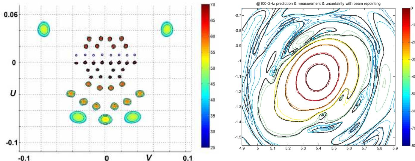
Uncertainty in the main beam shape after ground test campaign (integrated power, in percent of total) as a function of angular radius from peak.
