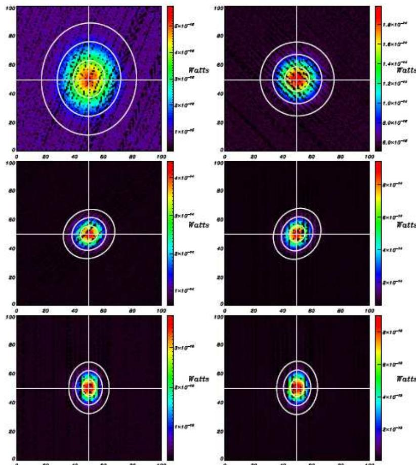
**Figure 23.** Maps of Mars, for the 100-4a, 143-2a, 217-6b, 353-1, 545-2 and 857-1 detectors, along with the best-fit Gaussian beam. Note that the motion of Mars is taken into account. The stripes visible here are due to the spacing between successive rings, which is a significant fraction of the FWHM of the beam.
