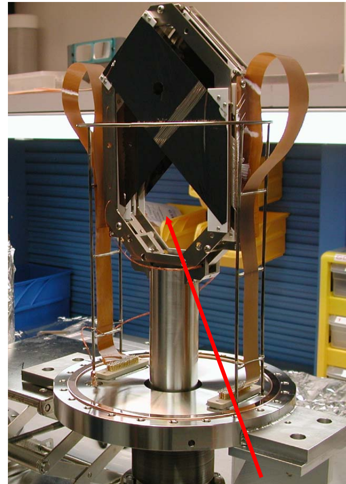
Beam hole for "detector out" position
