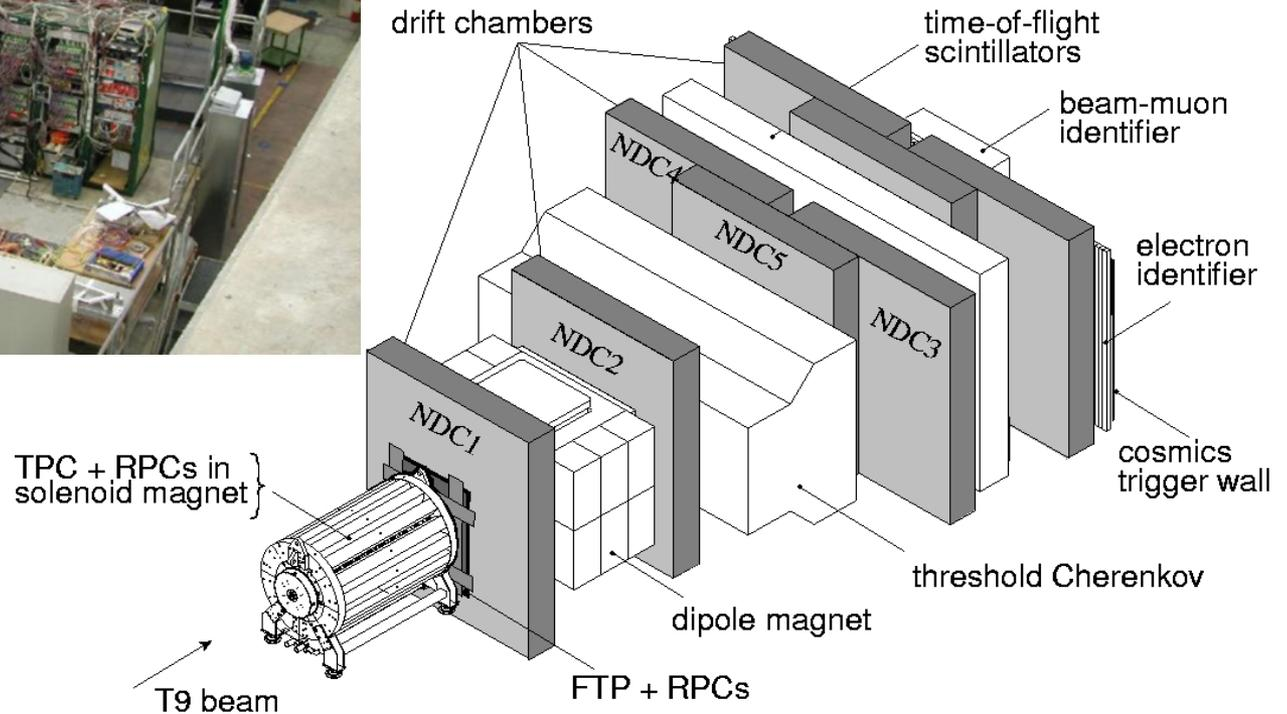
HARP: barrel spectrometer (TPC) + forward spectrometer (DCs) to cover the full solid angle, complemented by particle-id detectors
