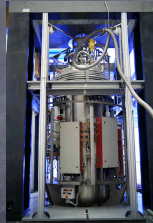
Warm bore cryostat for magnet
