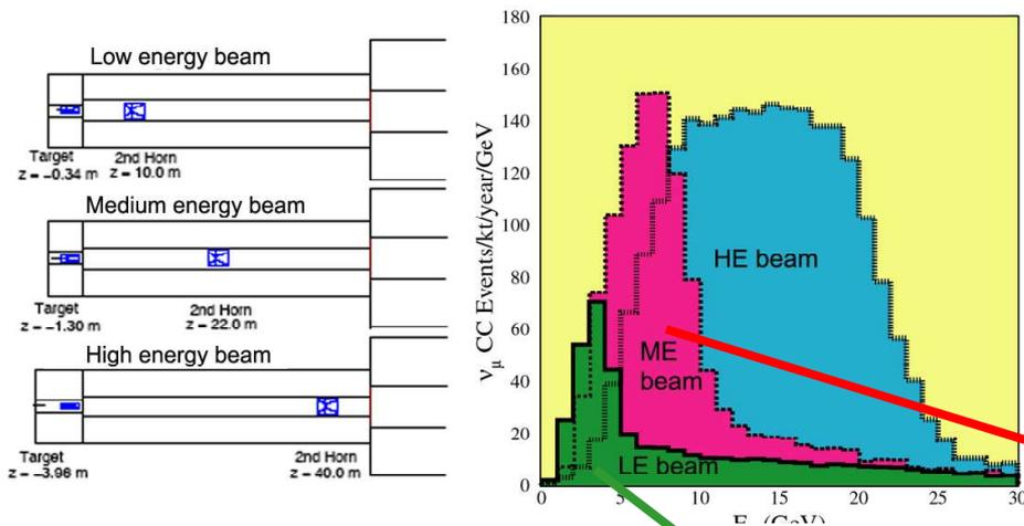
Can select low, medium and high energy beams by moving horn and target
