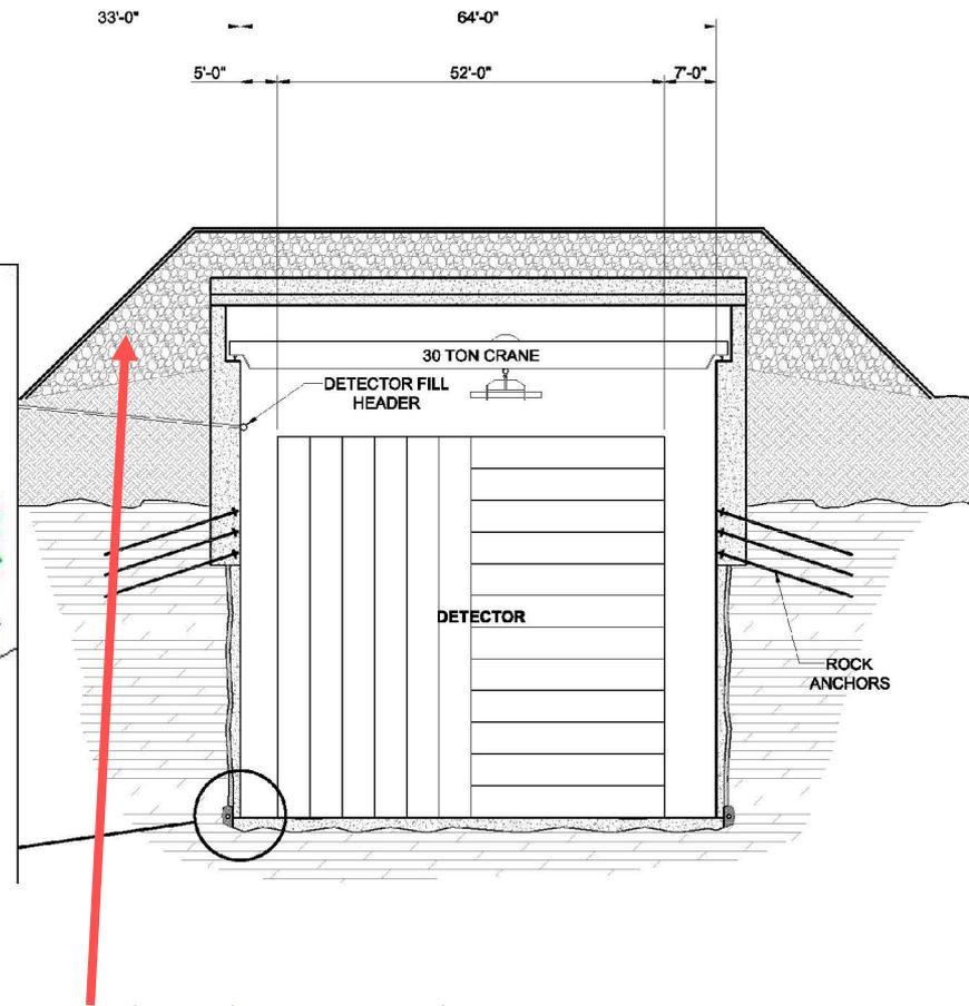
Surface detector with about 3m overburden to reduce
